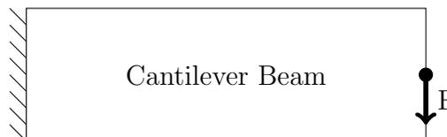
Figure 2.4: Cantilever beam boundary condition definition
