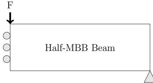
Figure 2.3: Half-MBB beam boundary condition definition
