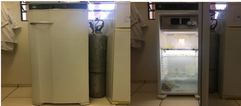
Figure 4. Schematic and pictures of BOD Refrigerator used as growing algae cultures under controlled environmental conditions
