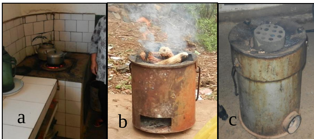
Figure 1: Stove types. a) Chimney stove with the chimney built into the wall of the house (n = 25). b) Portable bucket stove (n = 9). c) Portable stove for coal honeycomb briquettes (n=3).
