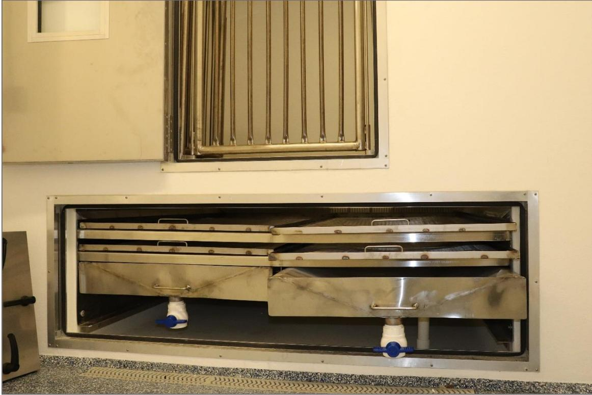
**Figure 3.7.** Secondary section of the calorimeter chamber.
