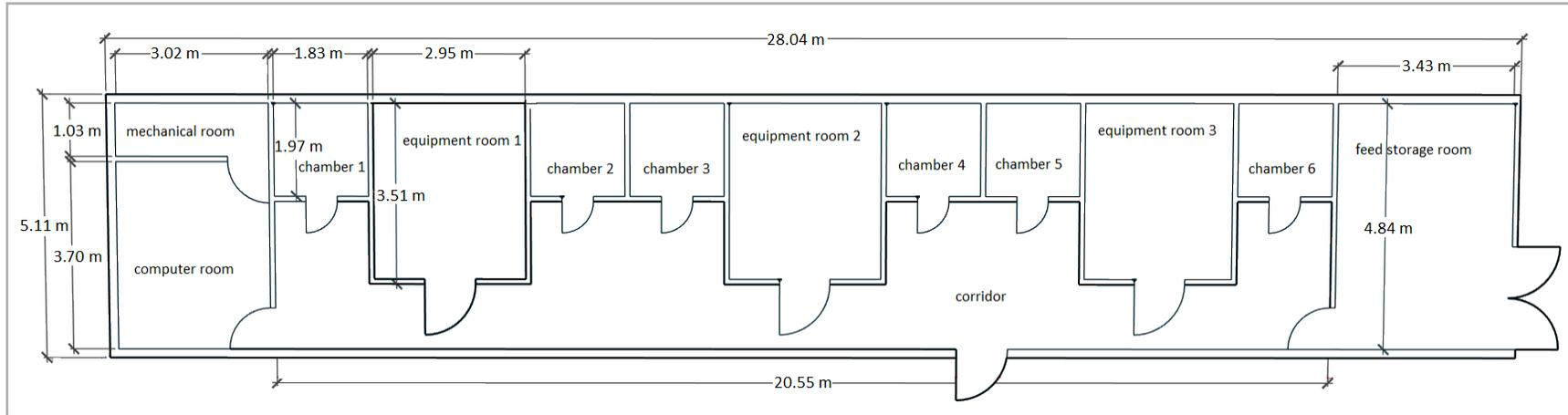
**Figure 3.1.** Layout of the swine calorimeter unit.
