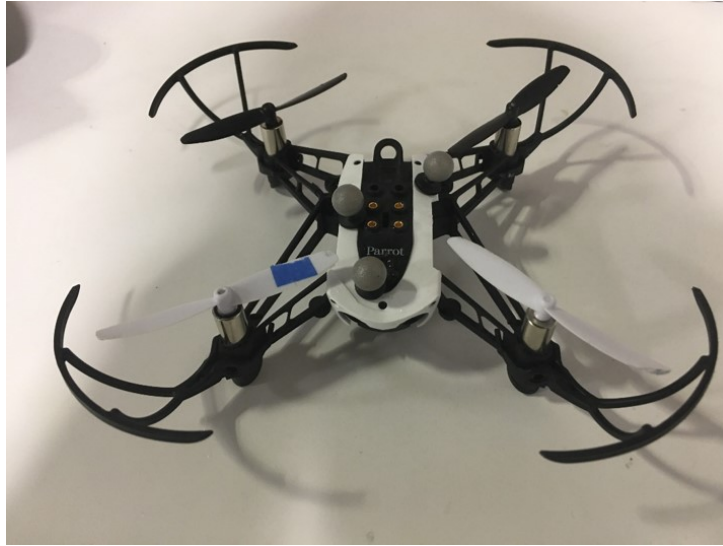
Figure 1.1: Parrot mambo mini drone fitted with vicon markers
