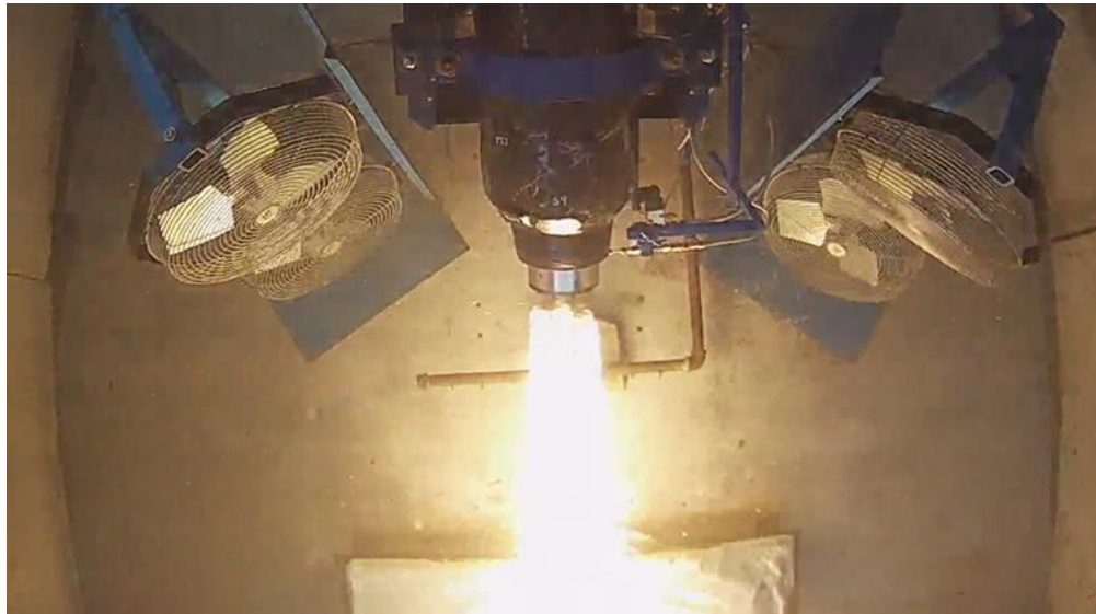
Figure 1 SPG Testing with Composite Case
