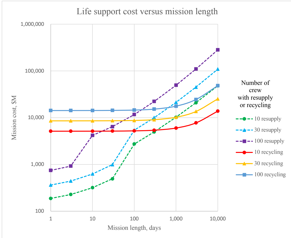
Figure 3. Life support cost versus mission length for a launch cost of 0.01 $M/kg ($10 k/kg).
