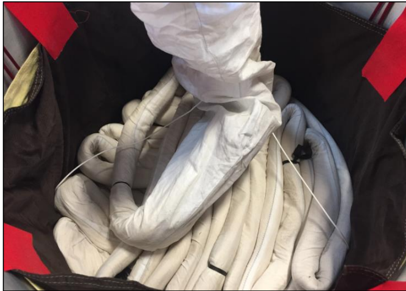
Fig. 5 Sensor activation lanyard in Drogue parachute.
