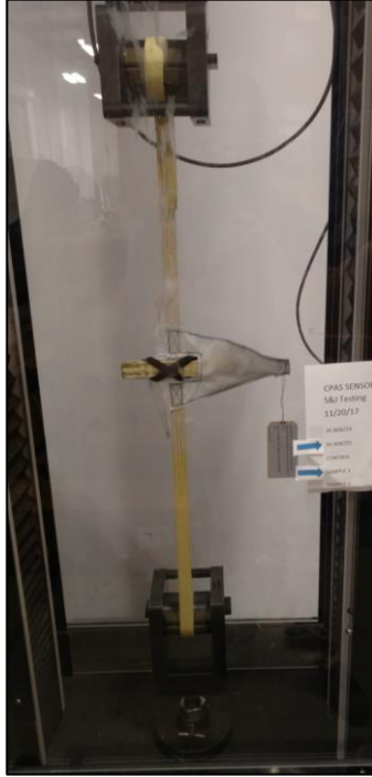
Fig. 6 Sensor pocket seam and joint testing.
