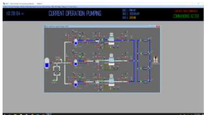
NPAS Autonomous Operations of the nitrogen system at the SSC High Pressure Gas Facility
