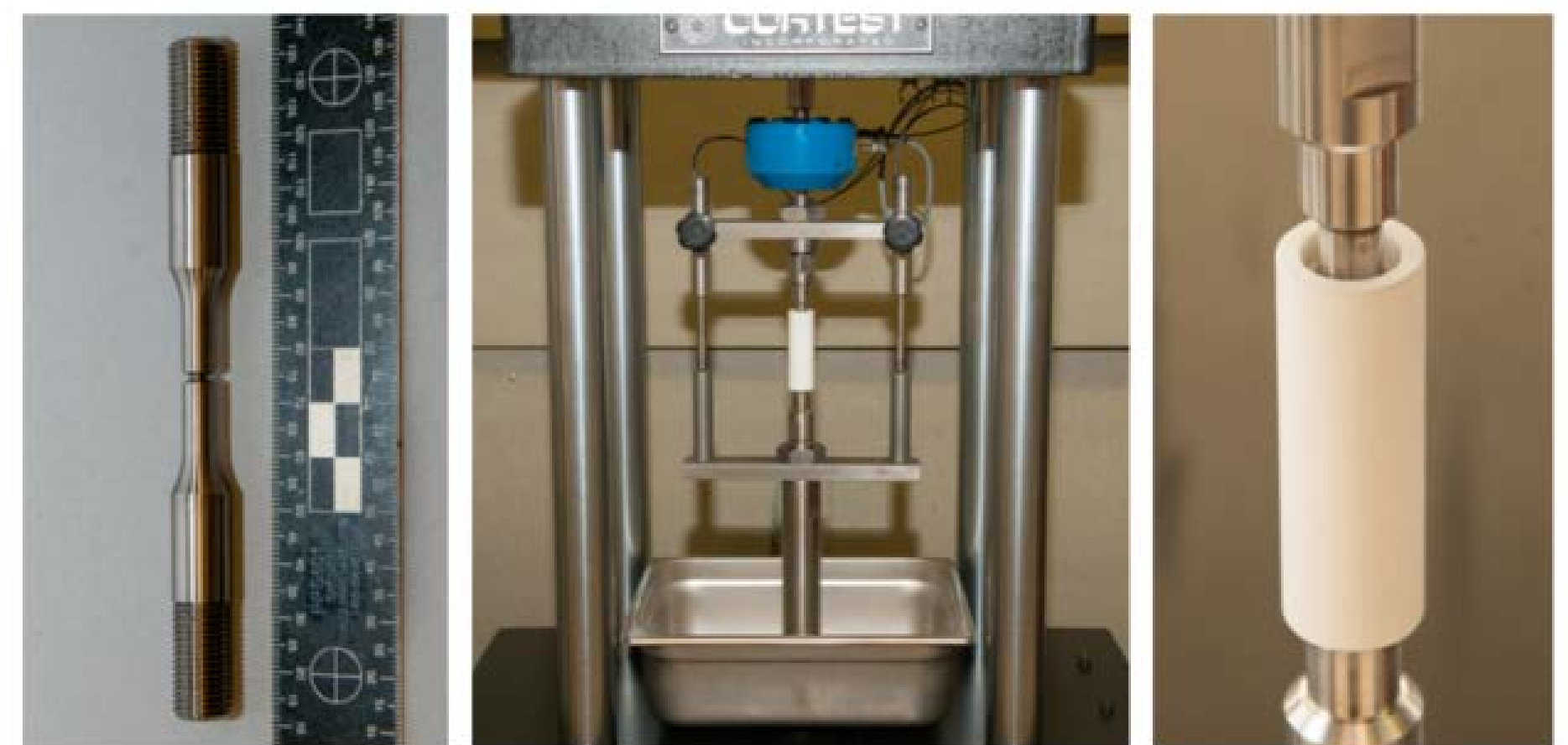
Photos: Pre-test specimen (wstf2018e20280), slow strain rate test in progress (wstf2018e20273), PTFE environmental chamber designed and used for oxidizer exposure (wstf2018e20277)
