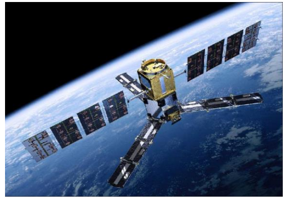
Fig. 1b. Large 2-D Aperture Synthesis Antenna (SMOS example)
