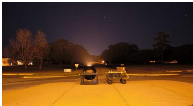
Figure 3. Initial deployment of Ground-based Accurate Active Light Source (AALS) for radiometric calibration of the VIIRS DNB's High Gain Stage (Image Credit: Robert Ryan NOAA-SBIR/IIR, Inc.).
