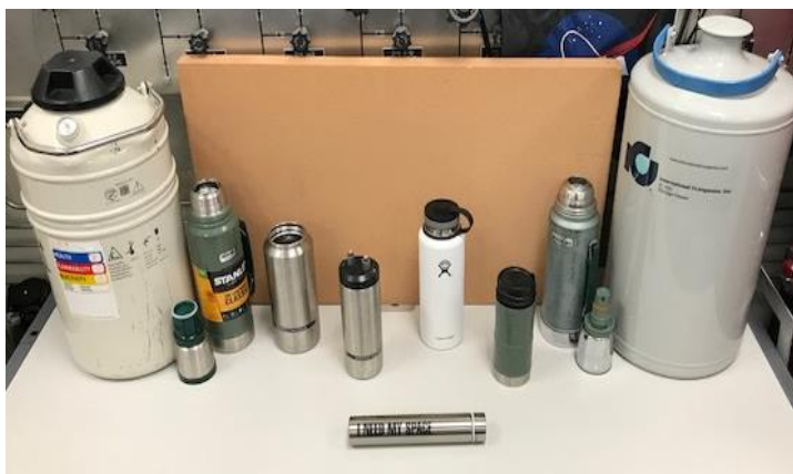
Figure 8. Cryogenic vacuum-jacketed test vessels.
