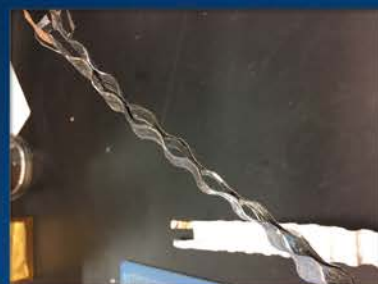
Corrugated honeycomb building block
