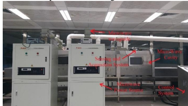
Figure 4. Tunnel-based microwave heating system
