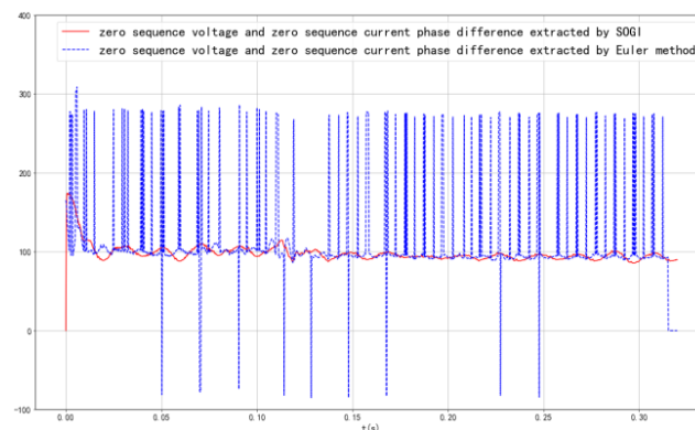
Figure 7. Comparison of phase difference extracted by SOGI and Euler
