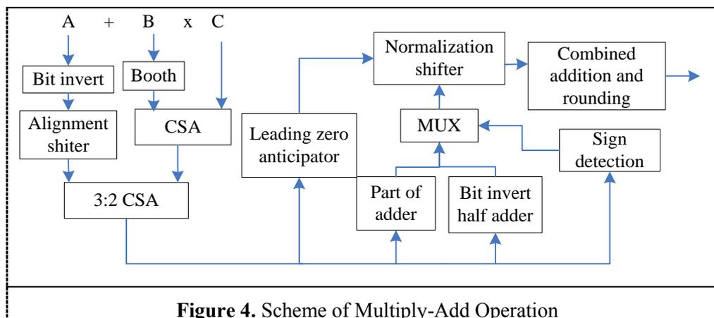
**Figure 4.** Scheme of Multiply-Add Operation
