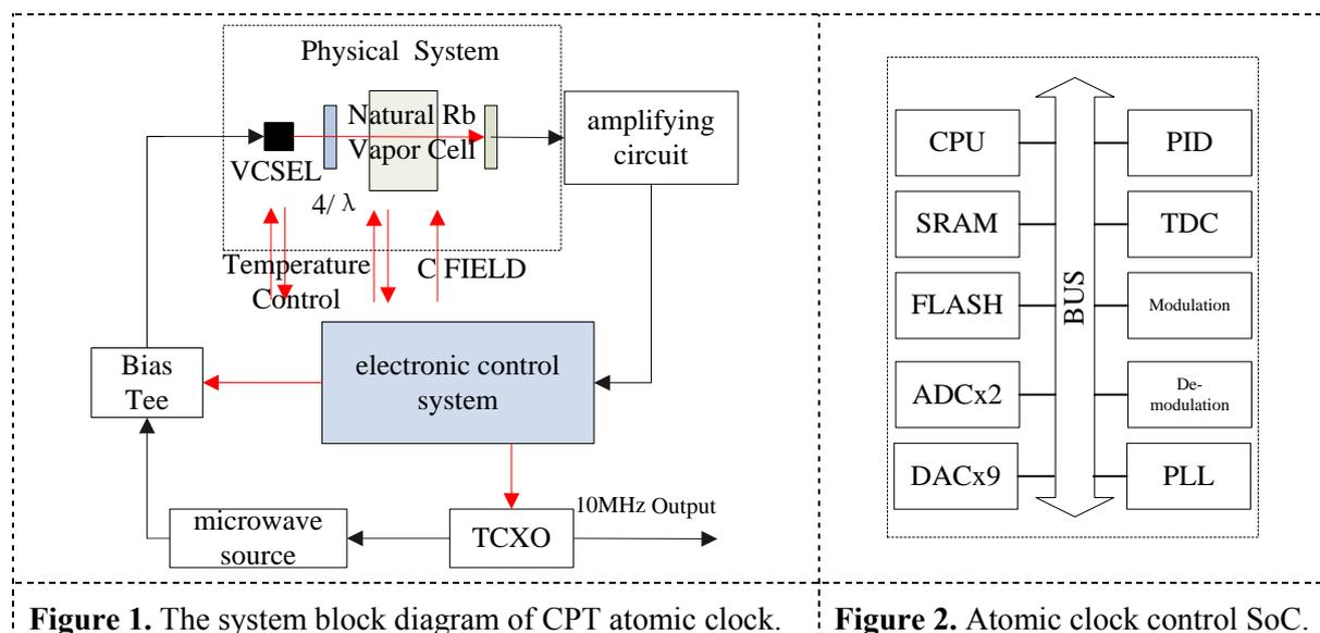
**Figure 1.** The system block diagram of CPT atomic clock.
