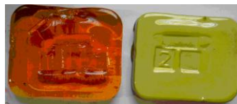
Figure 1. Enamel in ingots, transparent and opaque
