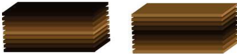
Figure 2. Schemes of forming a package of thermo-modified sheets of veneer.
