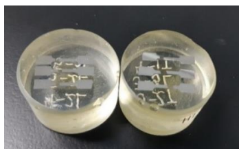
Figure 3. Tested miniature samples mounted in epoxy resin for microstructure analysis
