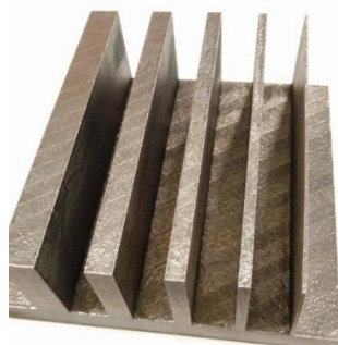
Figure 4. 3D printed part with different wall thickness.
