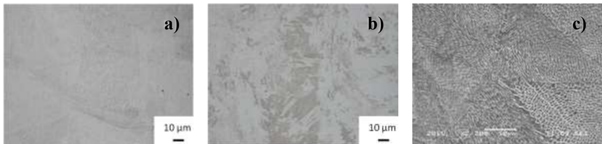
Figure 6. The maraging steel MS1 microstructure in as-built state (XZ plane) a) etched in Picral 4%, b) etched in a Vilella-Bain reagent, c) SEM image of the cellular structure with visible melt pools boundaries etched in Picral 4%
