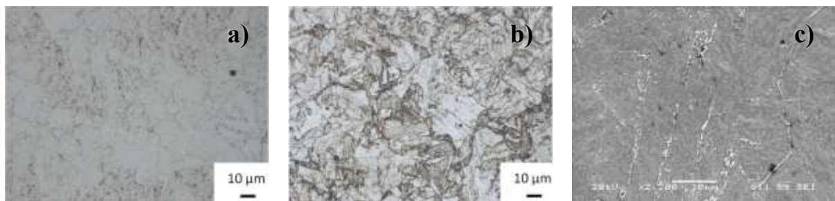
Figure 7. The maraging steel MS1 microstructure in heat treated state (XZ plane) a) etched in Picral 4%, b) etched in a Vilella-Bain reagent, c) SEM image of the structure with carbides precipitated along the grain boundaries
