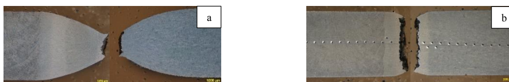
Figure 2. Macrographs of specimens creep tested at conditions: a) 575°C/200MPa/1345h and b) 600°C/80MPa/21294h.
