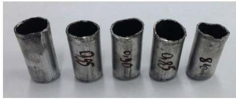
Figure 5. Examples of cylindrical drawpiece without collar made from EN-AW 1050A aluminium at coefficient of deep drawing m_d = 0.83 with different wall thickness obtained in experiment.
