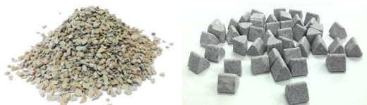
Figure 2. Zeolitic shapes with gradation 4-8 mm and ceramic media CB 20T
