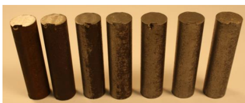
Figure 3. Steel samples a) without machining, b) after 60 min of treatment, c) 120min, d) 180 min, e) 240min, f) 300min and g) 1000 min
