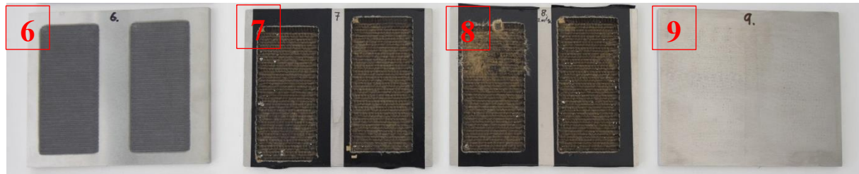
Figure 3. Sheets 6-9 after LSP treatment
