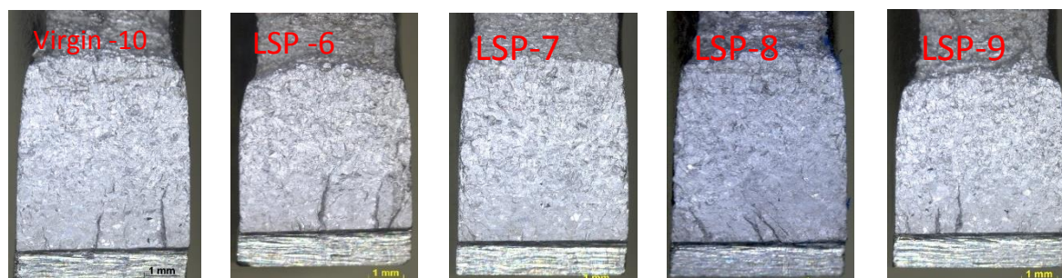
Figure 6. Fracture surface after HCF testing specimen from sheets 10, 9, 8, 7 and 6.
