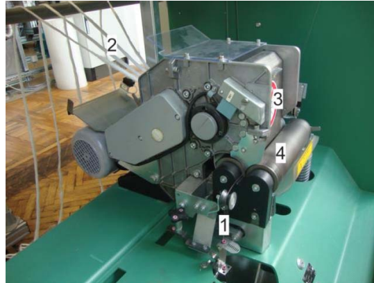
Fig. 2. Spinning head of the DREF 2000 friction spinning machine for the production of friction-spun SMA-HY (1: core feeding, 2: sheath feeding, 3: opening roller, 4: spinning drum) [11].
