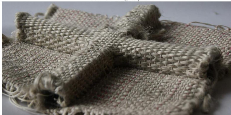
Fig. 4. Flaxen prototype of the 3D fabric based on a combination of a flat textile and two intersecting tunnels with rectangular cross-sections
