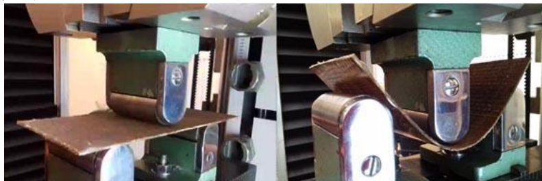
Fig. 5. Three-point bending test of a flat laminate
