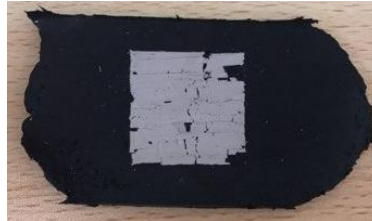
Figure 7. Sample with conductive silicone and PE 825 conductive ink.
