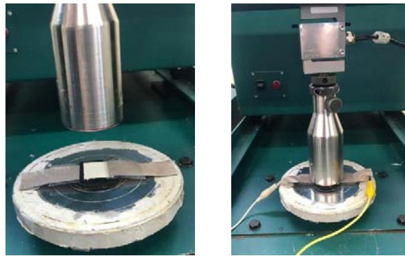
Figure 2. Compression test setup.
