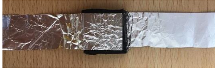
Figure 10. Sensor with conductive silicone and aluminum foil.
