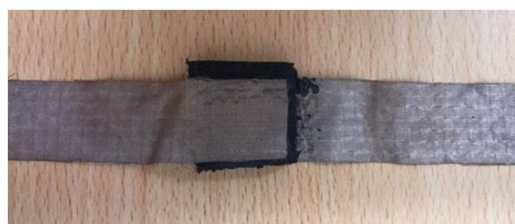
Figure 9. Sensor with conductive silicone and conductive fabric.
