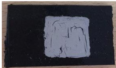
Figure 8. The sample with conductive silicone and PE 828 conductive ink.
