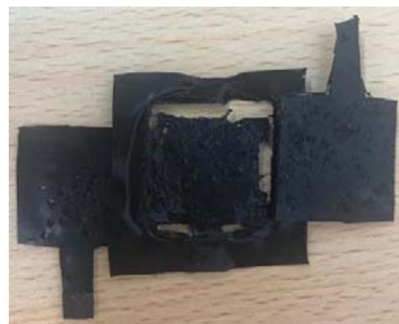
Figure 6. Destroyed sample prepared by hot press.
