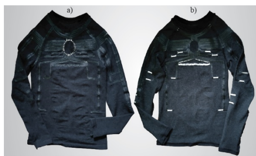
Figure 3. Shirt's prototype: a) exterior and b) interior
