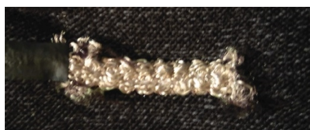
Figure 2. Knitted electrodes
