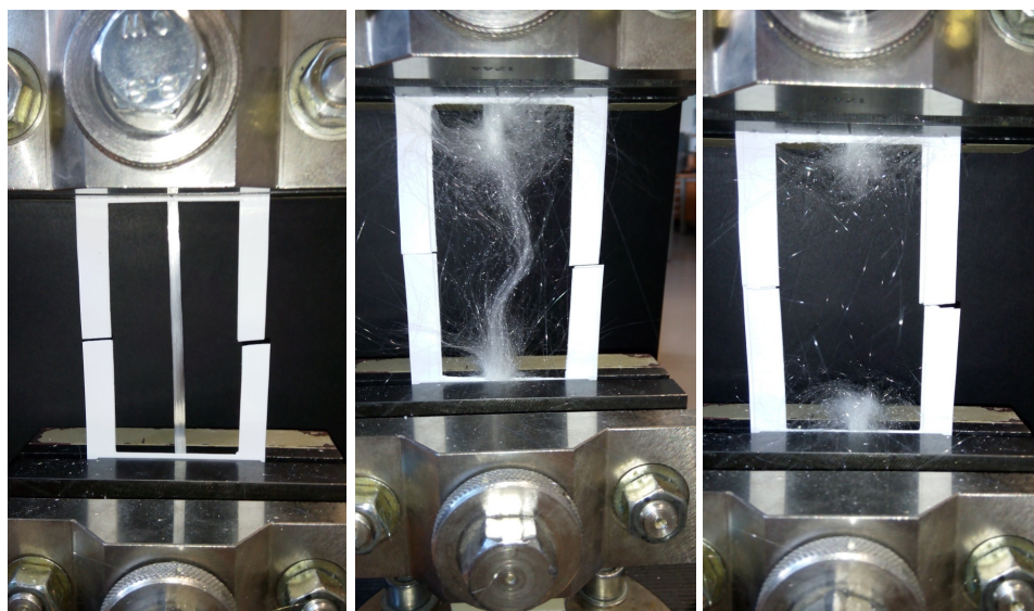
Figure 3. Behaviour of Glass roving in process tensile testing
