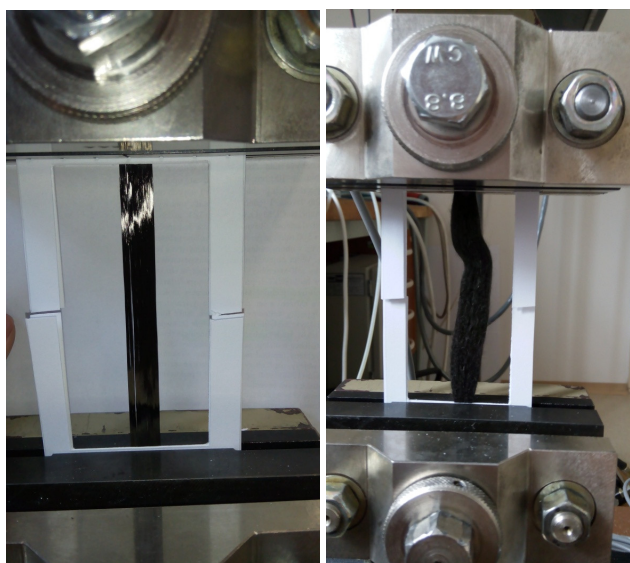
Figure 4. Behaviour of Carbon roving in process tensile testing
