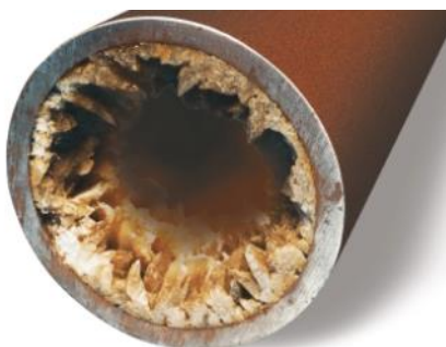
Figure 1. Pipeline with constricted diameter due to scale deposition [1]
