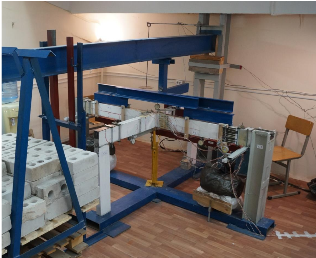
Figure 1. General view of the test reinforced concrete space frame.
