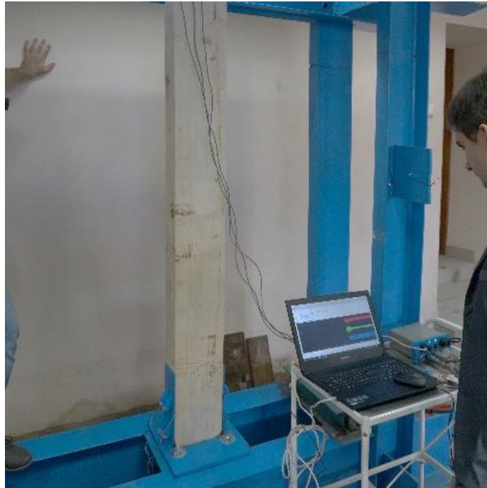
Figure 1. General view of the laboratory installation used to determine the natural frequency of the wooden column.
