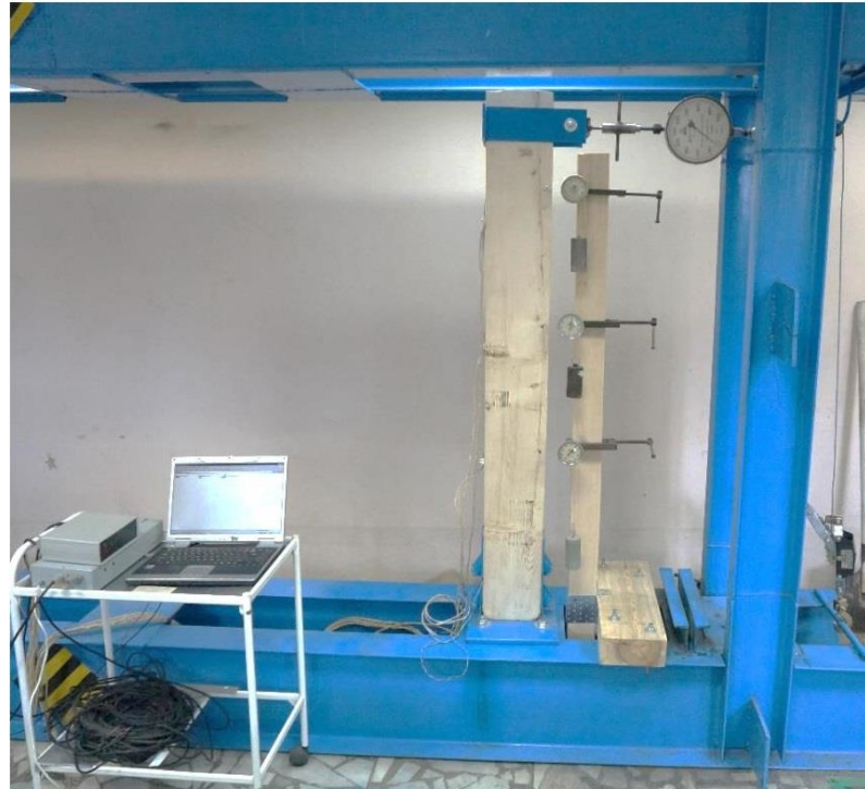
Figure 2. Scheme and general view of laboratory installation in static tests; 1, 2, 3 are the deflectometer number; P is the load.
