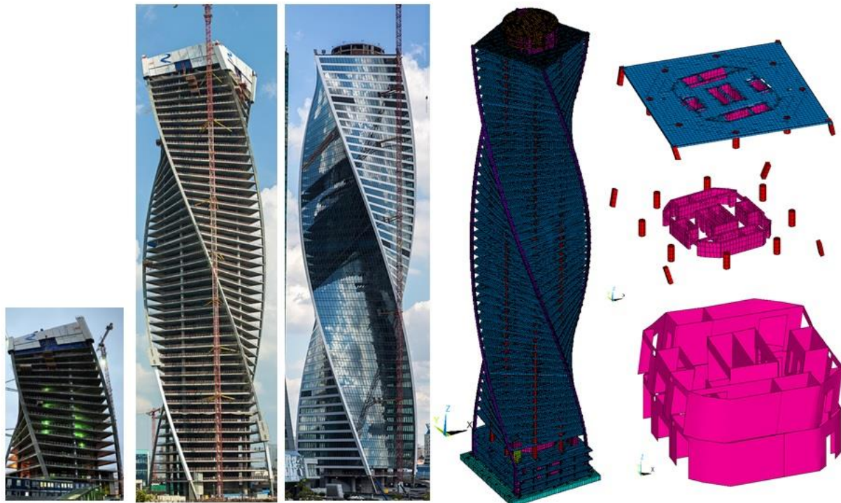
Figure 2. Elements of computational studies of the stress-strain state, strength and stability of the load-bearing structures of the “Evolution” tower of the “Moscow-City” complex with allowance for the actual position of reinforced concrete structures: construction stages and finite element models.
