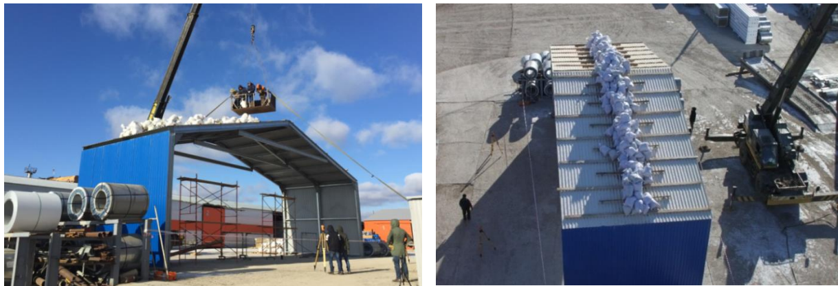
Figure 2. View of the frames testing block and a loading process.
