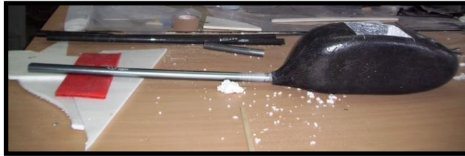
Fig .8 tail boom joined with fuselage
