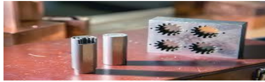
Figure 1. Different intricate shapes on(WEDM )
