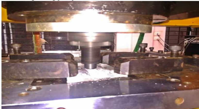
Figure 1. Friction Stir Welding Experimental Setup (With permission from NIT, Trichy)
