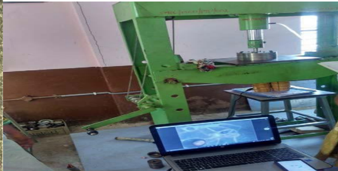
Fig 2 Formability test set up using hydraulic press and die.
