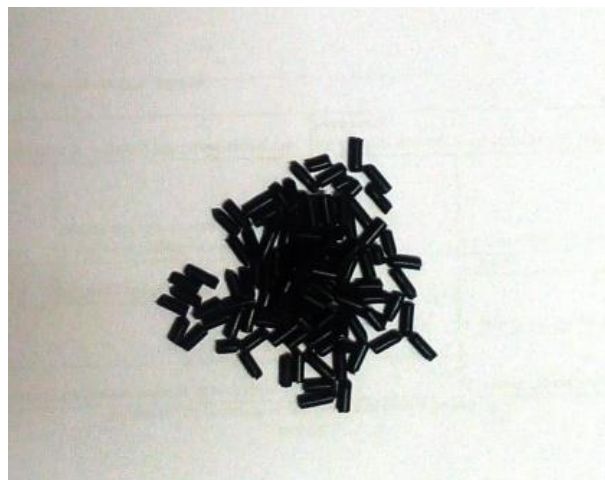
Figure 3: ABS dispersed with MWCNT pellets.
