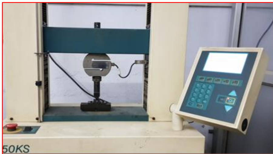
Fig. 2 Computerised UTM, H50KS on which the SBS tests were performed
