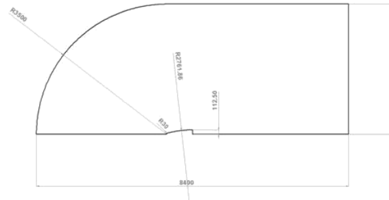
Figure 3. Geometric model of a ogival shape nose with domain
