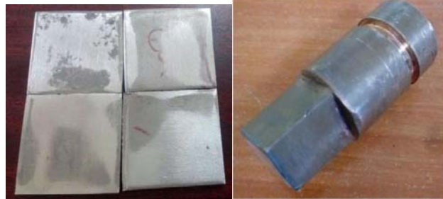
Figure1. Work piece Inconel 601 Figure2. Electrode material (Electrolytic Copper)
