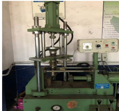
Figure 5.1: Hydraulic Plastic Injection Moulding Machine
