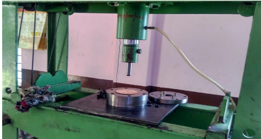
Fig.1. Formability test using hydraulic press and die fabricated as per to BIS-IS 10175 standard
