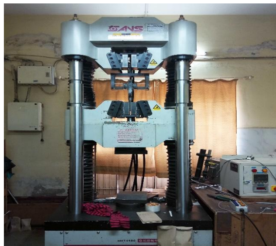
Figure 6. Flexural test machine
