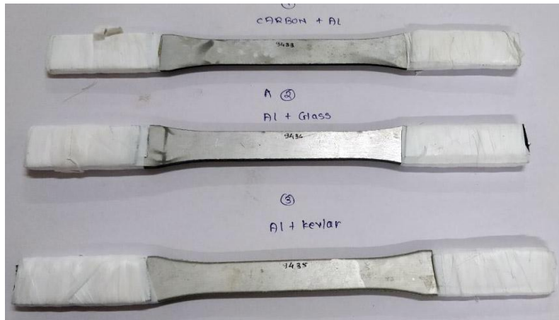
Figure 4. Tensile specimen
