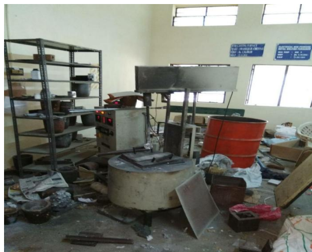
Figure 2: Inside View of Stir Casting Furnace
