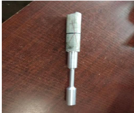
Figure 3: Specimen for Tensile testing as per ASME standards
