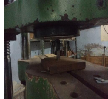
Figure 10. Compression testing
