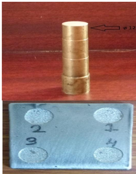
Figure 2. Machined surface of Inconel 601 using Brass Electrode.
