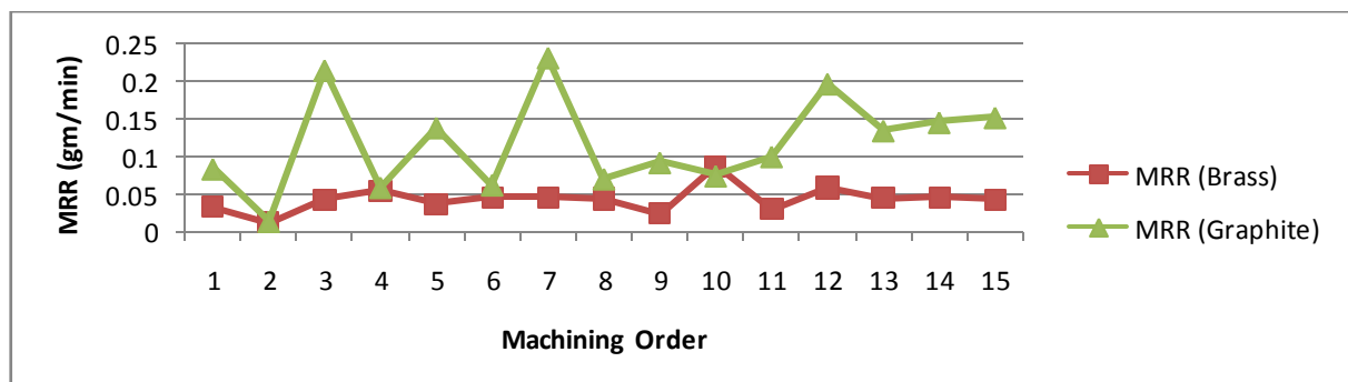
Figure 5. MRR comparisons with brass and graphite
