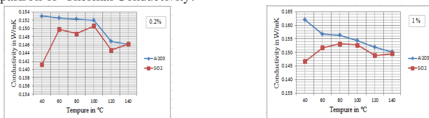
Fig 13: Comparison of Thermal Conductivity for Al 2 O 3 at 0.2% and 1% concentrations
